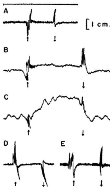
Fig. 2. Transverse voltages obtained under the conditions indicated in each case. Arrows indicate magnet movement as in Fig. 1. (A) Voltage measured from the electrodes alone with and without magnetic field. No d-c shift is observed ( 50 \mu\text{v}/\text{cm} ). (B) Example of the usual Hall voltage found in moderate anesthesia ( 100 \mu\text{v}/\text{cm} ). (C) Example of high magnitude Hall voltage noted during recovery phase of anesthesia; the two types of slow waves are clearly visible ( 100 \mu\text{v}/\text{cm} ). (D) Transverse voltage measurements after nerve section; no evident Hall effect is visible ( 50 \mu\text{v}/\text{cm} ). (E) Voltage after section of cord at medulla ( 50 \mu\text{v}/\text{cm} ).
