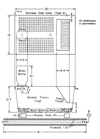
FIGURE 1. Apparatus employed to generate the power frequency electric field. A metal plate was permanently mounted between two sheets of plywood with provisions for applying and measuring the working voltage. Vibration isolation pads that supported the cage were glued to the upper wood surface.
